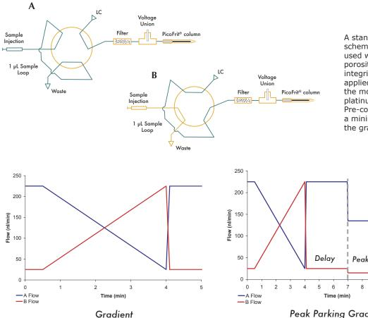
A standard 6-port injection scheme (1 µL volume) was used with in-line filtration (1 µm porosity) to preserve column integrity. ESI high voltage was applied pre-column directly to the mobile phase through a platinum wire micro-electrode. Pre-column volume was kept to a minimum ( $\leq$  1 µL) to minimize the gradient delay.
